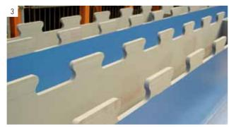
The steel girders were produced completely in the rolling mill including the corrosion protection. The approx. 32.5 m long girders were halved by a longitudinal cut of the web. This was carried out on a computerised machine, whereby three girders were machined simultaneously with three burner heads automatically in one cycle according to the stipulated recess geometry. The machining process guarantees a neat, low-distortion cut with excellent smoothness of the flamed surfaces.
